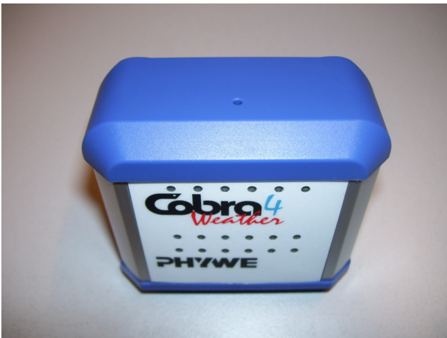
Fig. 2: Opening in the top for the light intensity sensor
